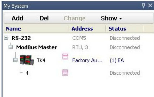
Selecting the unit address (4) enables Change button. To change the unit address, click the Change button on the tab or right-click on mouse to select Change.
