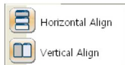
Chooses a screen align option from Horizontal Align and Vertical Align and aligns screens when multiple runtime screens (Data: Grid, Multi Panel, Panel, Line Graph, Bar Graph, Color Map Graph, Gauge Graph, Histogram Graph, Device: Alarm History Grid) are open.
