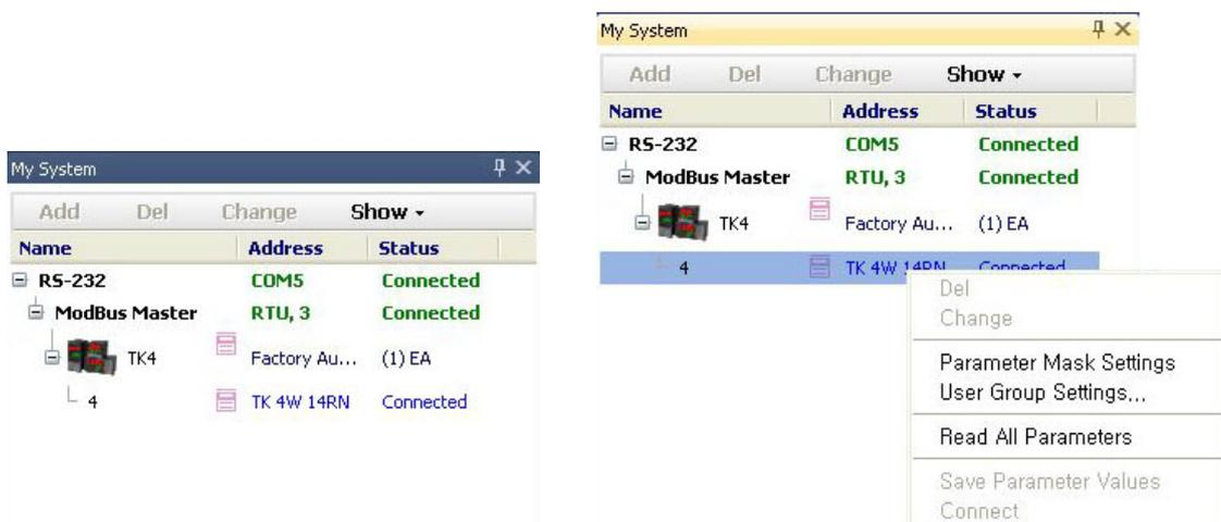
When the reading is completed, the Property window displays the parameters. Parameter change is also available.
