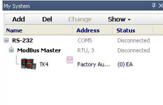
2nd When connected, select TK4 device, and right-click to select Scan Device.
