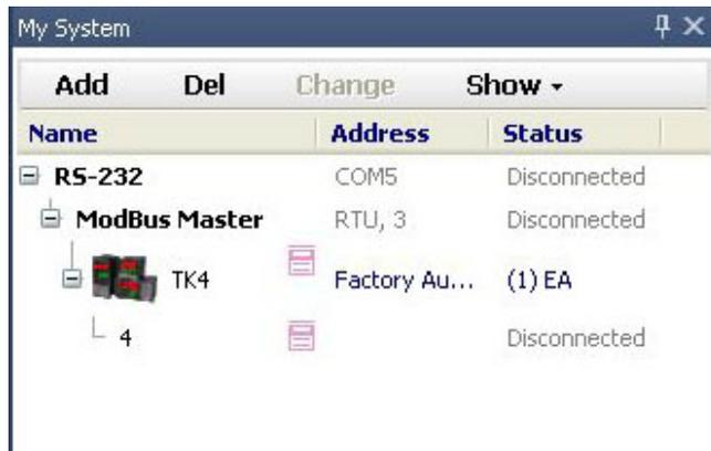
Selecting TK4 device enables Add button. To add a unit(address), click the Add button on the tab or right-click on mouse to select Add.
