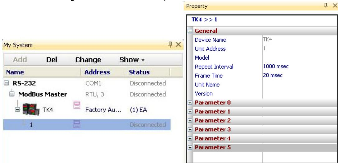
You can check and modify device parameters by reading parameters while connected.
